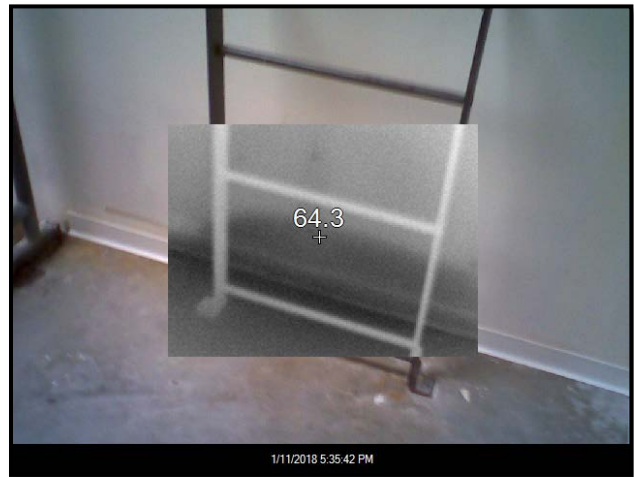
Photo 2: North Stairwell- East Wall (January 11, 2018) Thermal image of elevated moisture in drywall.
